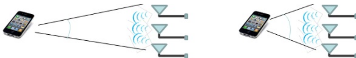
Figure 1. Narrower angular spread due to longer distance to the test antenna array (top left); wider angular spread resulting from proximity to the test antenna array (top right).
