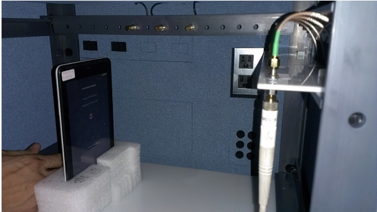
Figure 2. A handset (left) under test in a chamber that uses multiple MIMO test antennas (right).
