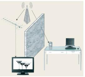
A hidden-node example signal from a TV station reaches WSD through a building or other obstructions and may be undetectable due to propagation losses. A TV antenna on the roof receives the same signal at a power level sufficient for viewing. WSD, not having detected the signal, may transmit and cause interference at the TV tuner.
