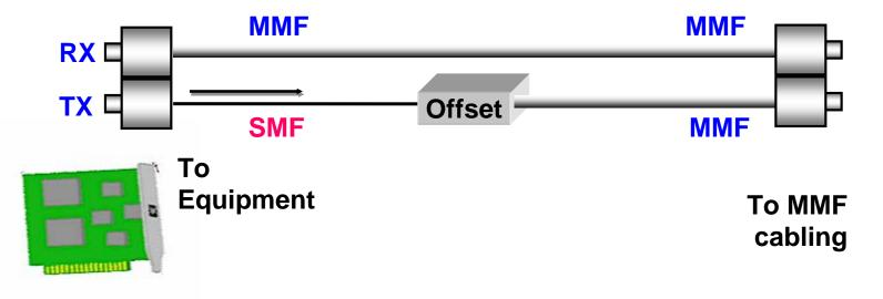
Offset patch-cord can be used with 1000Base-LX (1310 nm) gigabit Ethernet devices to address the DMD problem
