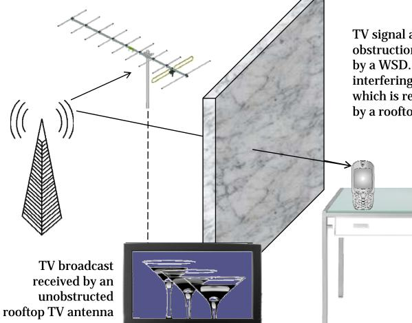
TV signal attenuated by an obstruction (wall) is undetectable by a WSD. WSD transmits, interfering with TV broadcast, which is received unobstructed by a rooftop antenna.
