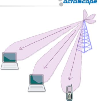
2x2 MIMO SM increases the peak data rate twofold by transmitting two data streams.
