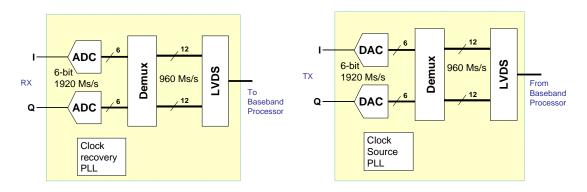
Figure 7: Radiospire ADC and DAC devices interfacing between the RF front end and the Baseband Processor
