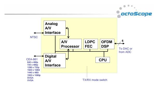
**Figure 6: Radiospire Baseband Processor** able to operate in either transmit or receive mode and interfacing between the video interface, such as the HDMI or the SVGA, and ADC or DAC chips
