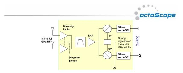
Figure 8: Radiospire RF Receiver device interfacing to the ADC
