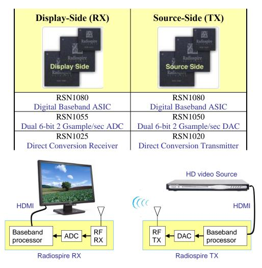
**Figure 5: Radiospire wireless HDMI solution** – UWB TX and RX. The video interface supports almost any standard format including HDMI, DVI, XGA and analog video such as NTSC, composite and S-video.
