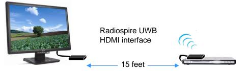
Figure 1: Testing verified studio grade performance of the Radiospire wireless UWB based HDMI cable replacement reference design.
