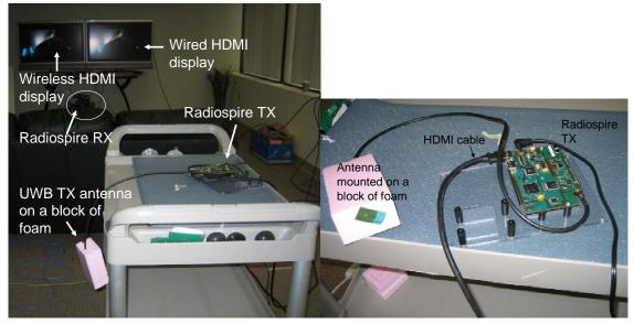
**Figure 10: Radiospire system test setup:** *left – transmitter with antenna hanging down and obstructed by the couch from the receiver; right – close-up of the Radiospire reference design*
