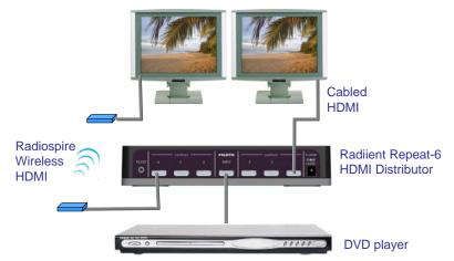
**Figure 2: Radiospire system test setup** – two displays side by side with one connected through an HDMI cable and the other via the Radiospire UWB link. The Radiient repeater was used to split the HDMI signal into two identical synchronized streams.
