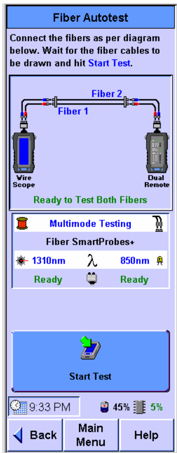
Figure 6: Screen shot from the WireScope 350 field tester showing the test configuration for two-way testing.
