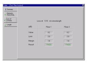
Figure 3: A sample test report displaying application-specific pass/fail results for each fiber optic network (left) in addition to the generic TIA and ISO pass/fail results for cable loss (right).
