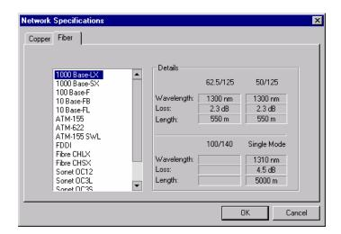
Figure 2: An example of fiber optic network test limits programmed into a field tester.
