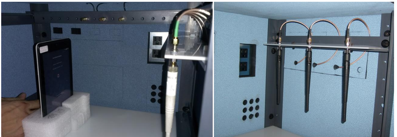
Figure 9: Example of MIMO test antenna arrangement inside octoBox small anechoic chamber. The MIMO antennas are spaced approximately the same way as they would be on an access point. All corner brackets and antenna rails are made of non-reflective plastic.
