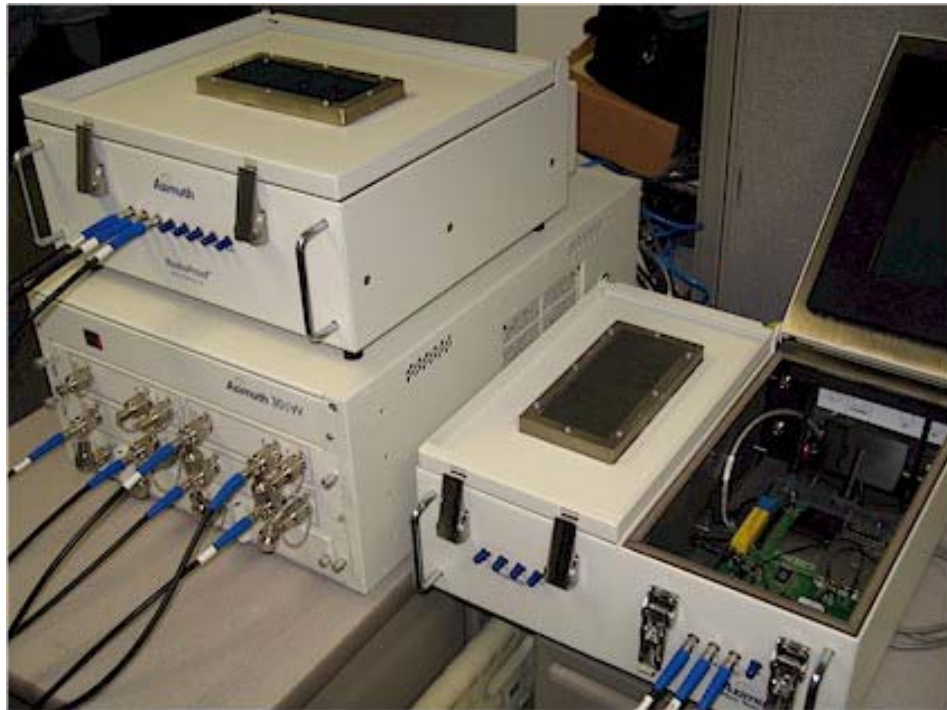
Figure 19: Azimuth 300W chassis and RPE-based conducted test setup for MIMO interoperability and throughput testing. Devices under test are enclosed in MIMO RPEs and connected through RFMs in the chassis.
