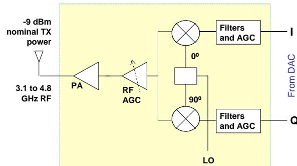
Figure 9: Radiospire RF Transmitter device interfacing to the DAC
