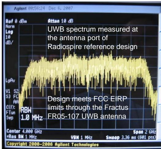
**Figure 4: Informal FCC compliance verification** – conducted spectrum measurement at the antenna port of the transmitter. The average power at the antenna port is below -40 dBm/MHz and with some isotropic losses through the antenna meets the FCC limit.
