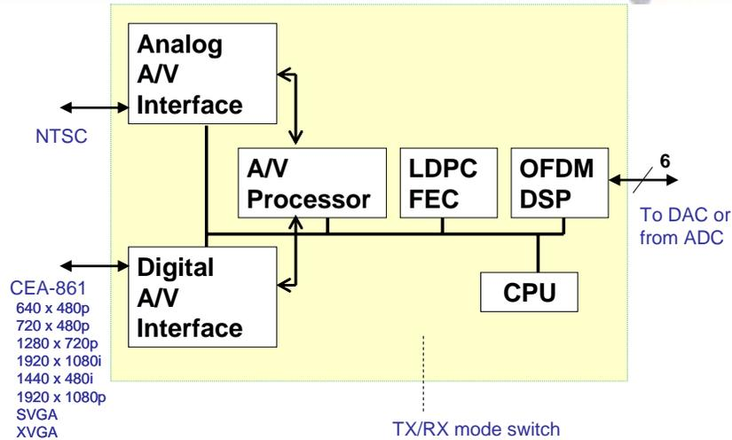
**Figure 6: Radiospire Baseband Processor** able to operate in either transmit or receive mode and interfacing between the video interface, such as the HDMI or the SVGA, and ADC or DAC chips
