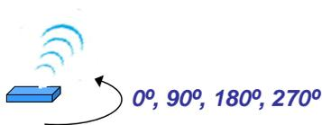
**Figure 11:** Video quality test was performed at 4 orientations of the cart with the transmitter rotated 0°, 90°, 180° and 270° with respect to the receiver. The antenna itself was also rotated and pointed up or down.
