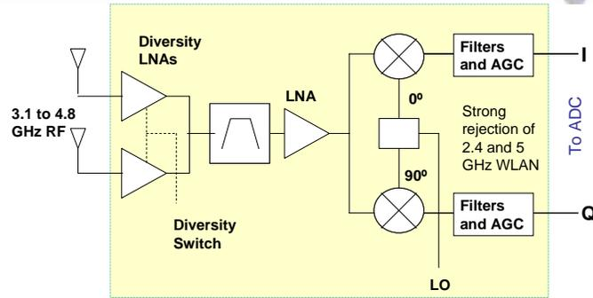
Figure 8: Radiospire RF Receiver device interfacing to the ADC
