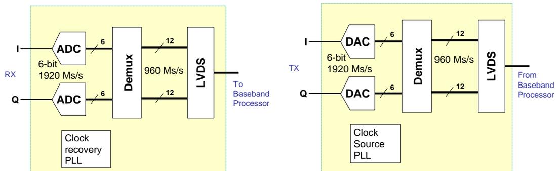
**Figure 7: Radiospire ADC and DAC devices** interfacing between the RF front end and the Baseband Processor
