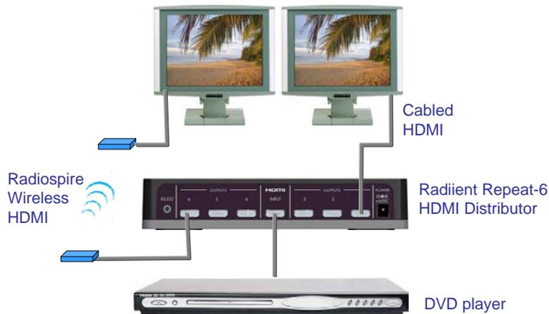
**Figure 2: Radiospire system test setup** – two displays side by side with one connected through an HDMI cable and the other via the Radiospire UWB link. The Radiant repeater was used to split the HDMI signal into two identical synchronized streams.
